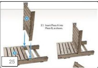
2) Insert Piece A into Piece B, as shown.
